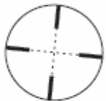
Incorrect Right Cant
